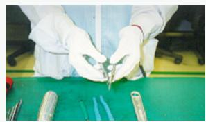
Handling modules near tools is prohibited because hard metal objects can damage modules.
