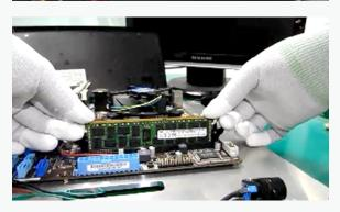
■ Do not insert DIMMs upside down. It can cause RTT resistor cracks.
