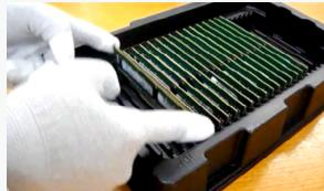
Modules should be picked up from packing trays only one-by-one.
