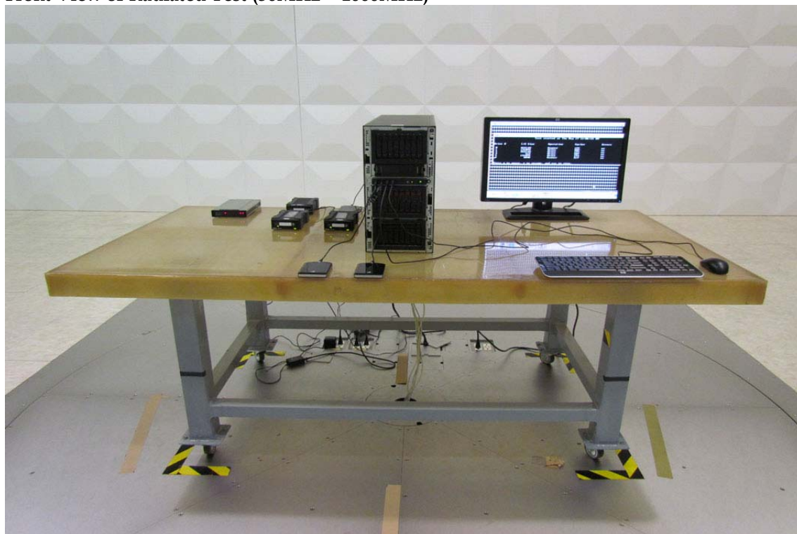
Front View of Radiated Test (30MHz ~ 1000MHz)
